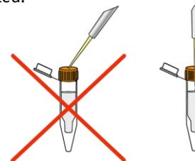
Insert pipet tip vertically through the hole in the column cap until forced through the lid valve (slight pressure release; otherwise, re-apply the pipet tip). Pipet the sample slowly (~5 sec) into the column.
