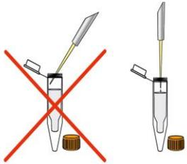
Open cap and pipet the sample slowly (~5 sec) onto the center of the resin bed of the prepared spin column. Close screw cap and loosen again half a turn.
