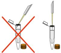
Open cap and pipet the sample slowly (~5 sec) onto the center of the resin bed of the prepared spin column. Close screw cap and loosen again half a turn. **Important:** Do not close the screw cap of the spin column tightly!
